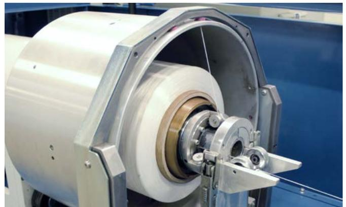
Tension measuring for binder head no. 2.
