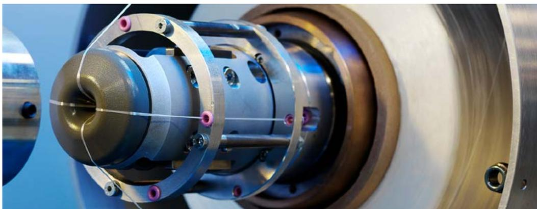
The torsion blockers secure that the SZ-stranded elements stay in position, while the cross-binding is performed in the single binding point.
