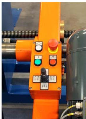
The pay-offs are operated by joy-stick or push bottom controls and the driving plate is available with a rubber carrier disc or carrier pintles.
