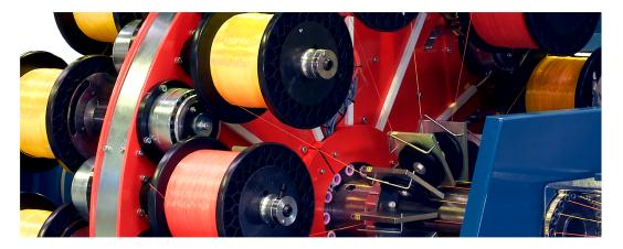
With this versatile server, tight-buffered fibers may be precision stranded in several layers on top of a central cable element.
